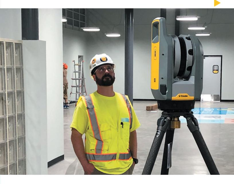
Trimble X7 3D Laser Scanner and Trimble FieldLink™ improve accuracy and facilitate collaboration between office and field
